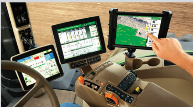
The new John Deere Connect Mobile app allows growers to monitor job quality in real time to better understand their sprayer or planter detail. (Photo: John Deere)
