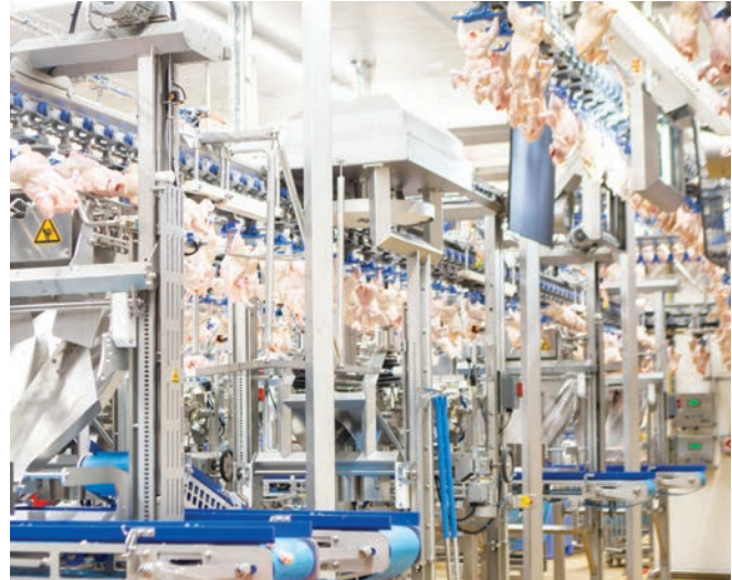
The IRIS camera system is seen to visually assess the quality of the wings in the line.
