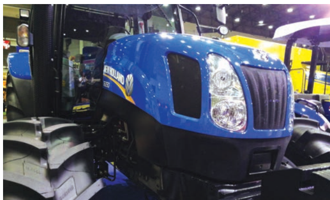
T6050 has a 128 hp 6.7-litre six-cylinder diesel engine with intercooled turbocharger.
