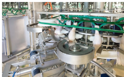
The Meyn frame for the Flex Plus cut up system is an overhead-mounted cut up frame for supporting cut up modules. (Photo: Meyn)
