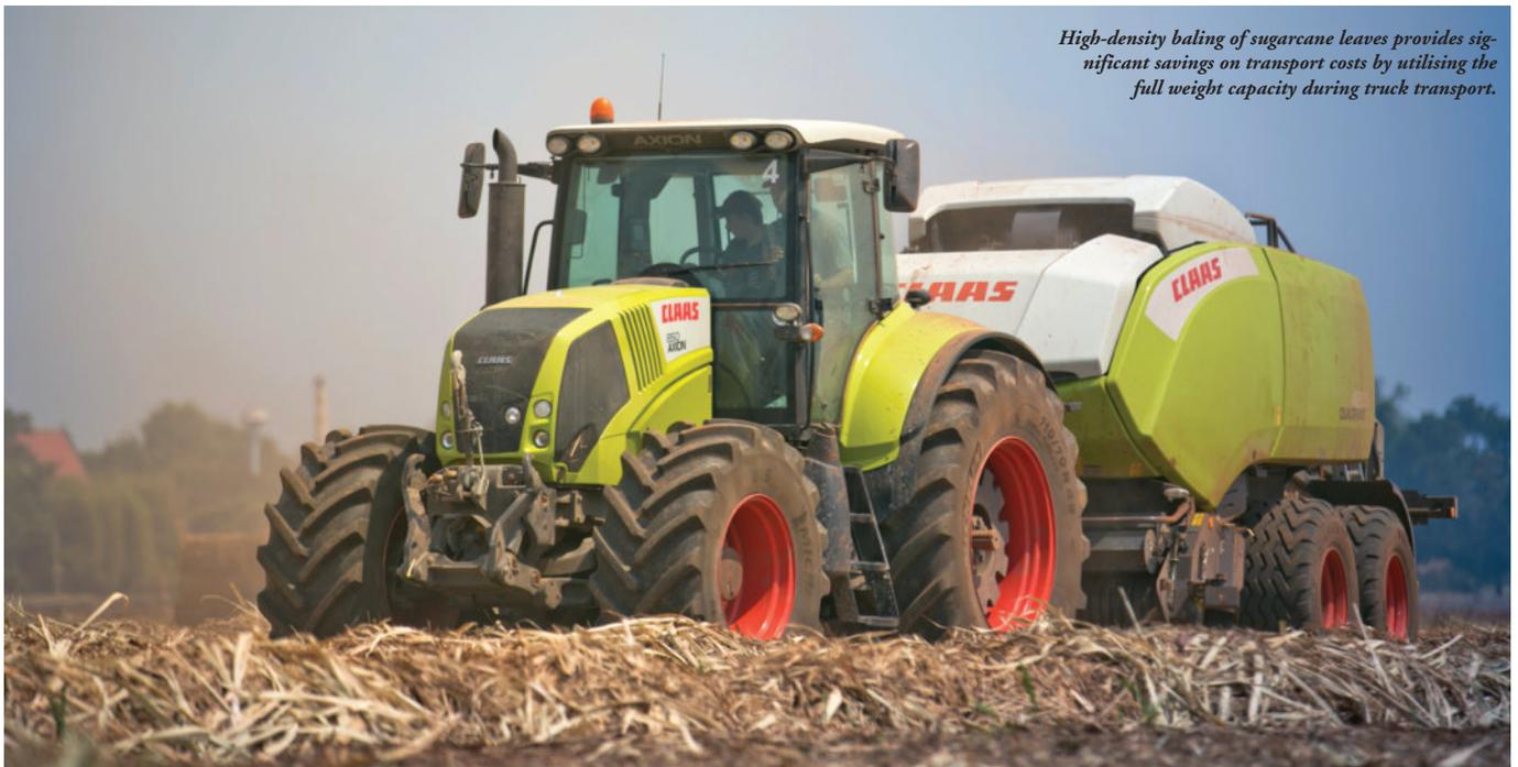
*High-density baling of sugarcane leaves provides significant savings on transport costs by utilising the full weight capacity during truck transport.*
