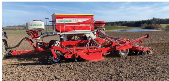
Seed distribution on the TEGOSEM is pneumatic.
