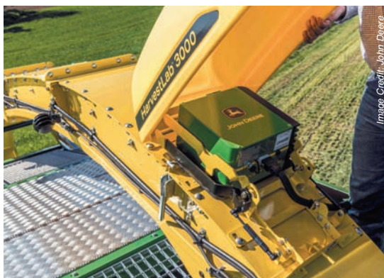
When mounted to John Deere self-propelled forage harvesters, HarvestLab 3000 can monitor forage constituents at harvest.
